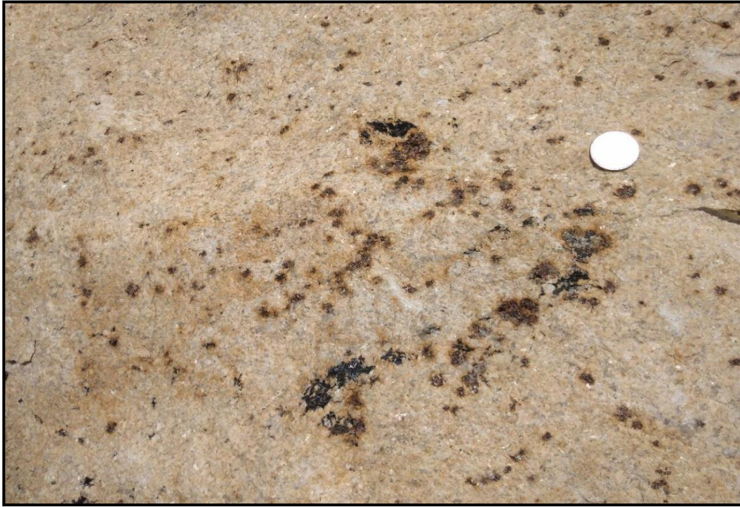
Presence of sporadic garnets and biotite reduces the quality (Latt. 10^{\circ} 3'57.10 and Longi; 78^{\circ}25'3.80'' )
