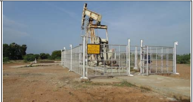
Sucken Rod Pump mechanized oil well near Greater Kovil Kalappal, Thiruvarur District (Location: 10°34'03.21"N 79°31'50.18"E)
