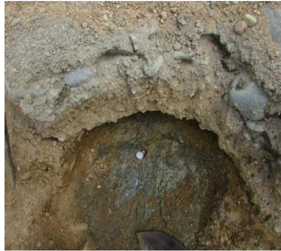
Photo: 30. Pits excavated in the river course (R.Then Pennar) for removing the top gravel containing gold grains, Edathanur area, Loc. Edathaur and collecting weathered material for panning., Loc. Edathaur
