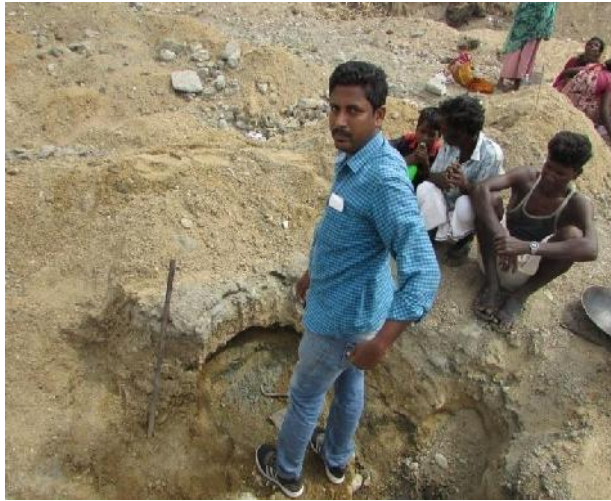
Photo: 30. Pits excavated in the river course (R.Then Pennar) for removing the top gravel containing gold grains, Edathanur area, Loc. Edathaur and collecting weathered material for panning., Loc. Edathaur
