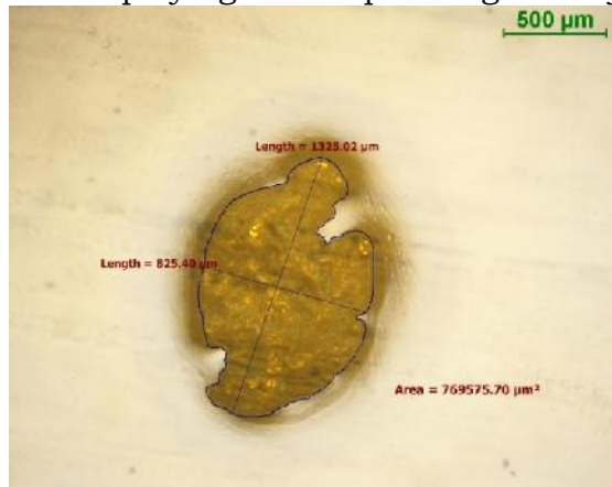
Photo: 52 - 53. Photomicrograph of gold grains displaying the shape and geometry
