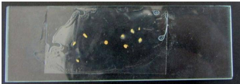
Photo: 41. Gold grains mounted on thin section
