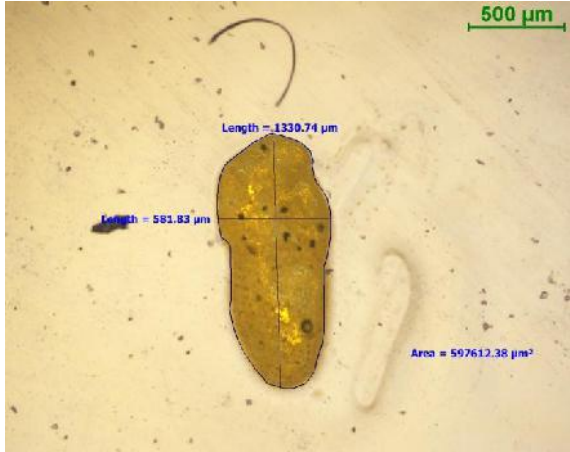
Photo: 50-51. Photomicrograph of gold grains displaying the shape and geometry
